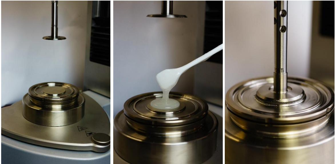
Figure 17: Measurement setup using a parallel-plate geometry
