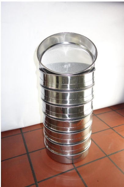
Figure 14: Sieve column.
